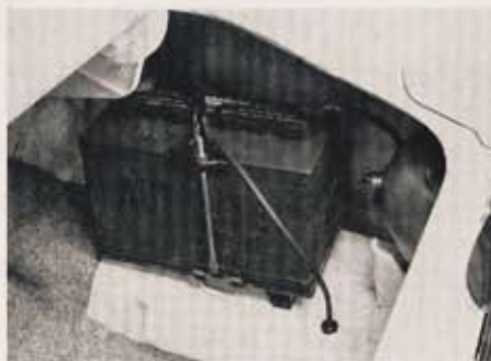
Above: Design of hood scoop is unique to the Boss 429. Right: Optional on other Mustangs, Magnum 500 wheels were standard on the Boss. Below: Battery was banished to the trunk because the engine bay was already filled with 429 cubic inches of fire and fury.
