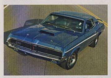
Hood scoops were painted body color on the '69 Eliminator, but were a contrasting matte black on the '70 model. They were not functional except with the ram air 428 CJ. Also, note that the Eliminator came with one racing mirror, remotely operated, on the driver's side. There was no side mirror on the passenger side.
