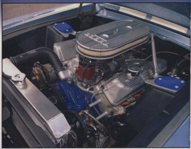
rockers. The original aluminum intake uses an 850 cfm Holley four-barrel carburetor. The ignition is from MSD. The engine was balanced and blue-printed. The engine produces 500 horsepower.
